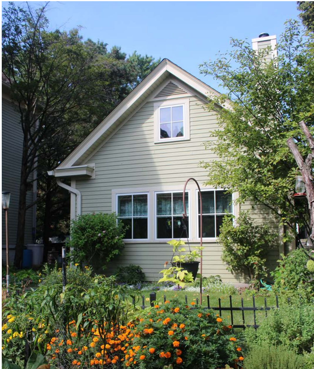
The casement windows on the ADU limit thermal bridging compared to the main home's double hung windows. The window's divided lite pattern relates to the main house as do the smaller details like the triangular gable louver vent and the fascia with crown molding.
